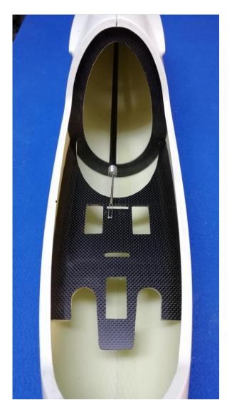
Mark a cardboard with the shape of the fuselage (canopy zone); use the cardboard shape to realize the plywood base (thickness: 5 - 6 mm.)
