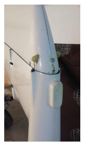
Install the steel cable inside the fuse and crimp it to the servo and to the rudder moving part
