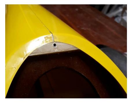
Make a hole behind the karman end insert a bowden as shown in the picture – glue it with epoxi 5 min.
