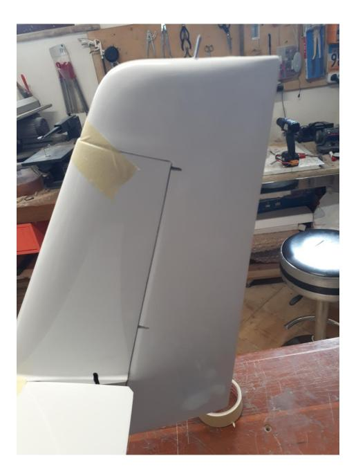
**GLUE THE RUDDER TO THE FUSELAGE WITH RESIN** (or UHU PLUS ENDFEST 300).
