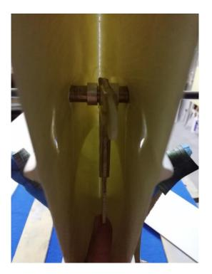
INSIDE THE TAILPLANE THERE IS A MAGNET ABLE TO JOIN IT TO THE STEEL BAR
