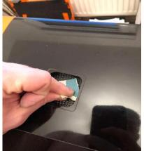
Sand the gluing surface
