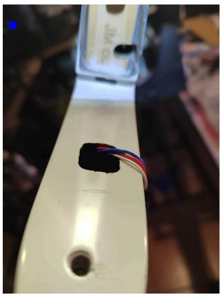
Rudder and elevator servo wire extensions must be long enough to reach the nose of the fuselage, using big section wire. Wire must be attached to the fuselage top either using american tape or wire holding platic clips, as you like. It is important to keep wire away from turbine heat.
