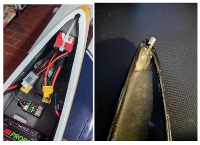
Install the specific fastening tool on the opposite side of the canopy. Open a window in the fuselage to pass the rod.
