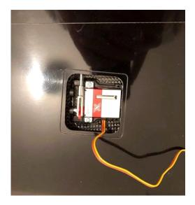
Solder the servo cable to the MPX connector (6 pins – male) following the scheme previously used for the female connector.
