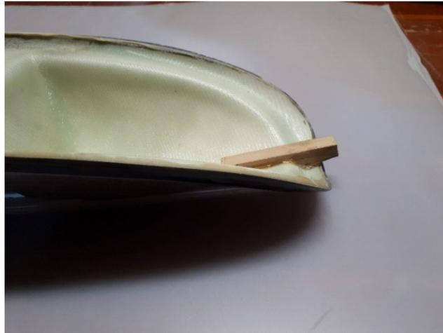
Make a slot in the front side of the fuse
