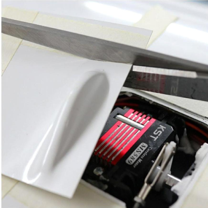
Join the servo cover to the wings with transparent tape
