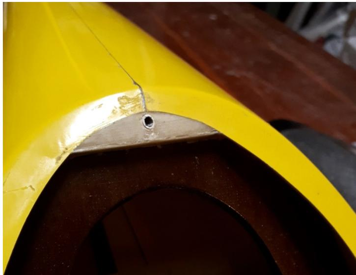
Make a hole behind the karman and insert a bowden as shown in the picture; glue it with epoxi 5 min.
