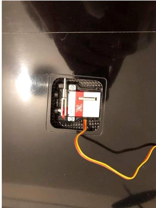
Solder the servo cable to the MPX connector (6 pins, male) following the scheme previously used for the female connector. Before gluing it to the wing, check the right connection (MPX male/female) of the wings to the fuse.
