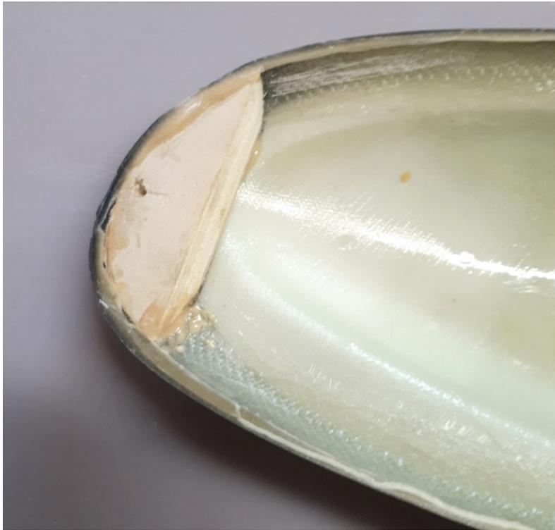
Glue a piece of plywood in the back side of the fuselage and make a hole (bowden diameter)
