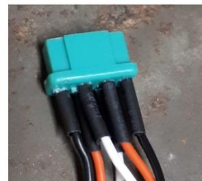
Now you can glue the MPX (female) connector to the fuselage
