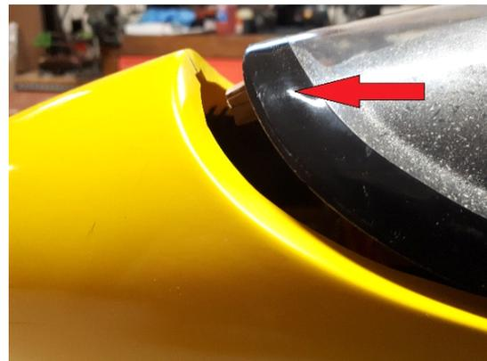
Glue (epoxi 5 min.) to the back side of the cockpit base a piece of plywood
