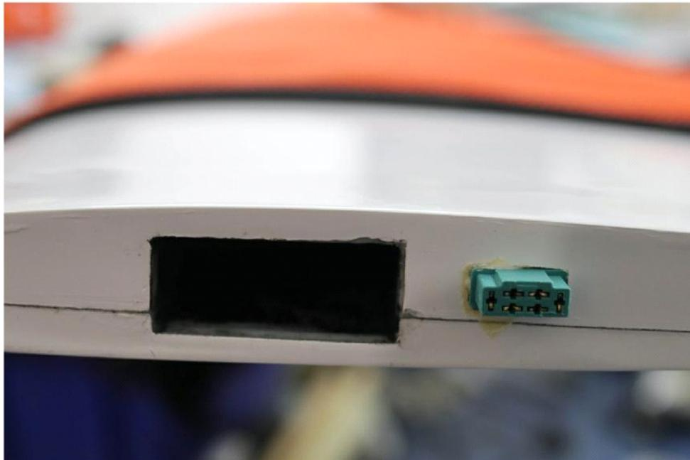
Put the servo cover over the opening, mark the cutting area with paper tape and remove with scissors the excess part
