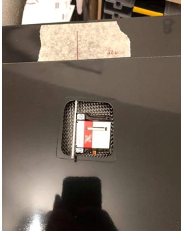
Mark the same axis position also in the upper side of the aileron; cut (with Dremel) the opening for control horn and cut the "nail" opening in the wings
